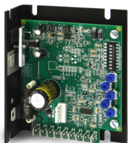
Low-Voltage Controls WPM Model 0786/0788 (12V or 24VDC)
