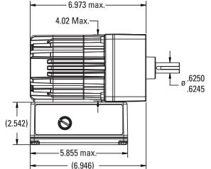
**Optional Accessory** Mounting bracket, model 0970 **Gearmotor Weight** approximately 9 lbs.
