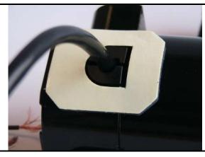
Remove the backing from one side of the foam gasket. Firmly press the adhesive side onto the motor cord strain relief.
