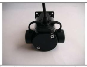
Firmly press the rubber cover against the adhesive foam gasket. Slide each end of the rubber cover onto the cast 'ears' of end shield.
