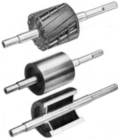
Fig. 2-20: Comparison of typical reluctance synchronous rotors (top) and hysteresis synchronous rotors (middle and bottom).
