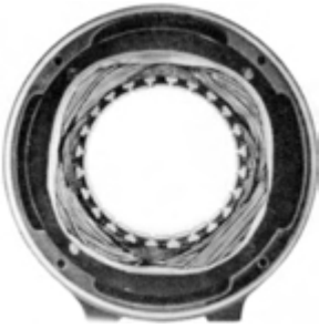
Fig. 2-11: Typical four-pole, split-phase stator.
