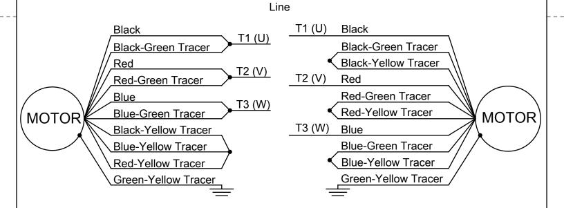
**Direction of Rotation: Clockwise** To reverse direction of rotation, transpose any two line leads.
