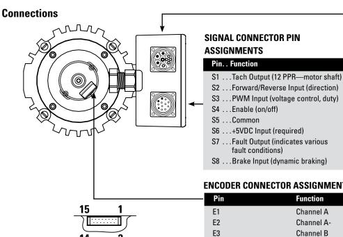
Three connections must be made. Two cables are required for the control box. The user also must provide and install a third cable for the optical encoder.
